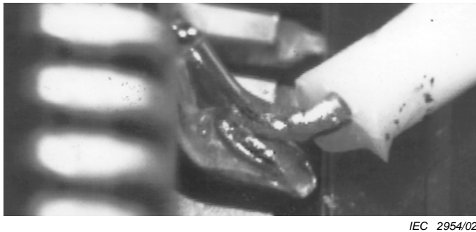
Nonconforming – Level A, B, C Fractured solder joint.
