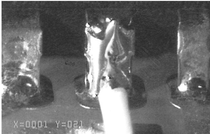
Acceptable – Level A, B, C Acceptable solder joint at wire.
